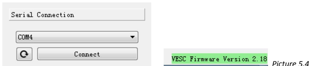
5.5 Choose Motor Configuration >> Motor and click Read Configuration. It will read the VESC settings and check if the parameters are same with the below picture. If it is not same, please revise the parameters, then click Write Configuration to download the new parameters.
